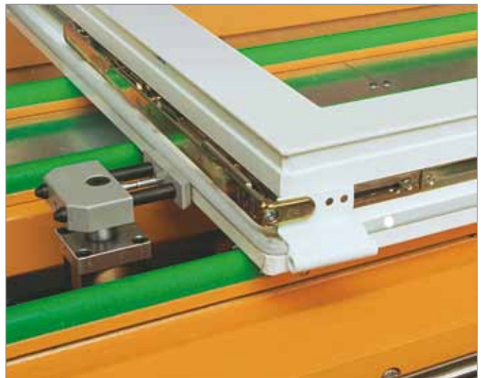
Reading assessment right and left, pneumatic lowering for the fitting-length calculation
