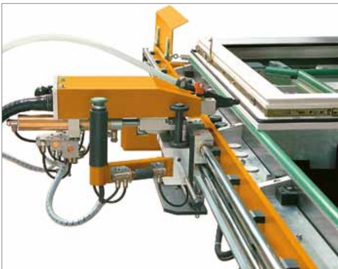
Mobile feeding-screwdriver with automatic screw feeder
