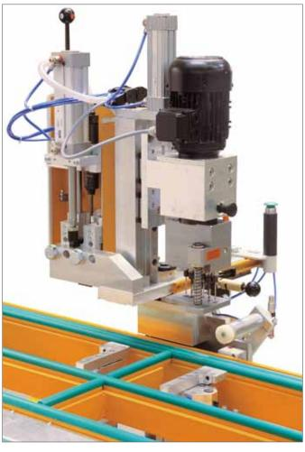
Two pneumatic fold stops that are lowerable below table height with a rotary turret for the exact positioning of two to four different frame construction depths
